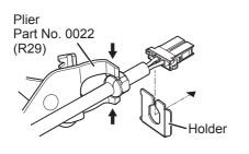
2. Release the pliers when the bush comes to the position shown in the figure, and the bush will be engaged in the holder.
