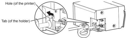
Attach the supplied cover to the printer securely using the supplied screw for securing the cover.
